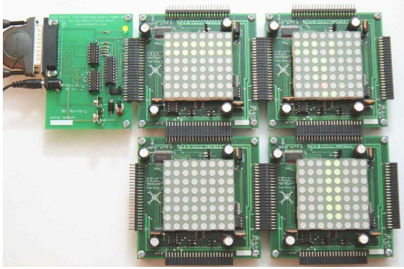
Figure 3. Four MOD 88 boards connected as a 32x32 Matrix A single PC Interface Board controls all four boards via the upper-left board, using the distributed control of the Cell Matrix architecture.
