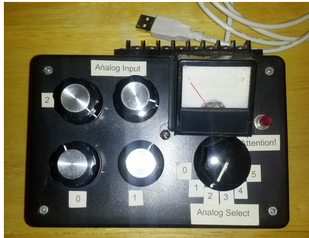
Fig. 1.29. Songline Processor Prototype. Analog inputs are specified with the knobs, while analog outputs can be read from the meter (the selector below the meter chooses which output channel is displayed). Software running on a USB-connected host machine emulates an 8 \times 8 array of 3-sided cells. 6-bit digitizing is used, resulting in a total function memory of 128 MB.
