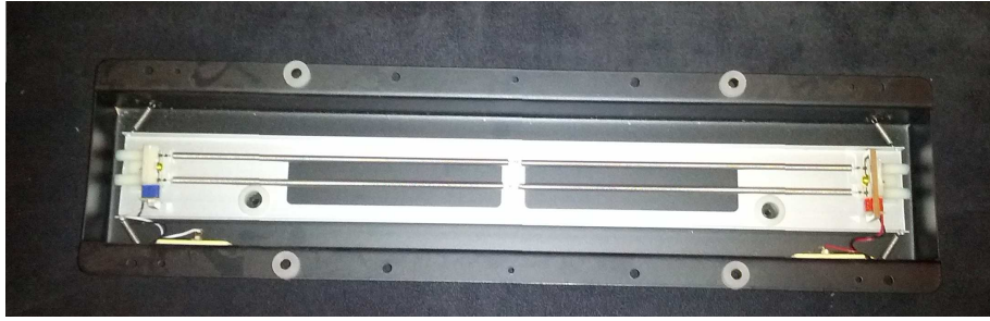
Fig. 1.24. Mechanical Spring-Based Delay Unit. An analog signal can be sent into one end of this unit, where it is transformed into mechanical motion that causes the springs to oscillate. The signal travels through the spring to the other end, where a transducer converts the mechanical motion back into an electrical signal, which can be amplified and re-sent to the starting point. This is one way to store an analog signal.
